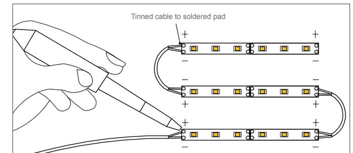
Please note drawings are an installation guide only. Each LED Ribbon Strip application may have variable factors. Cable size may need to be specified to limit the voltage drop throughout the circuit.
