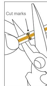
**To ensure IP66 rating:** All open LED COB ribbon ends need to be covered with a power connector or end cap. Do not leave any end exposed.
